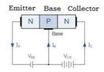
the negative pole of the battery and the p type base is connected to the positive pole of the same battery  $V_{\text{EE}}$
