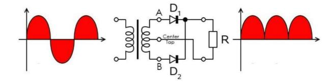
In the above circuit, two junction diodes are connected to a load. This circuit gives out in both positive and negative halves of the AC cycle. Hence, it is a Full-wave Rectifier. In this circuit, the p-sides of both the diodes are connected to the input. And, the n-sides are connected together and connected to the load.
