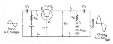
AC voltage gain (A<sub>V</sub>) = Output voltage / Input voltage
