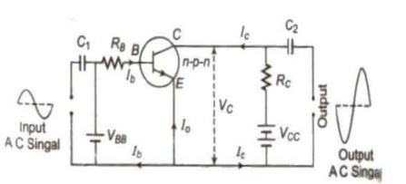
AC voltage gain  $(A_V) = B_{AC}$  \* resistance gain
