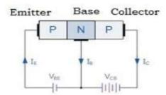
forward biased which means the p type emitter is connected to the positive pole of the battery and the n type base is connected to the negative pole of the same battery  $V_{\text{EE}}$
