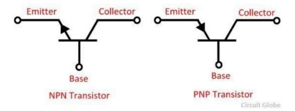
The arrow in the symbol indicates the direction of flow of conventional current in the emitter with forward biasing applied to the emitter-base junction. The only difference between the NPN and PNP transistor is in the direction of the current.
