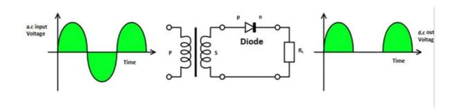
In the second half cycle, current will flow from negative to positive and the diode will be reverse biased. Thus, at the output side, there will be no current generated and we cannot get power at the load resistance. A small amount of reverse current will flow during reverse bias due to minority carriers.
